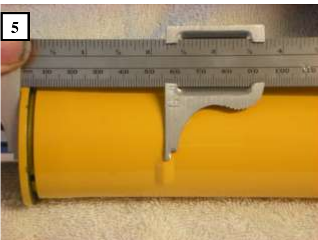
5) Measure the indentation on the Koni from the top of the strut. In this case, 50mm distance from top to the marking.
