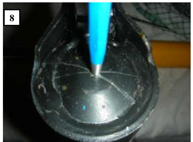
8) Using a punch, mark a hole dead center in the bottom of the strut housing. Drill a 14mm hole.
