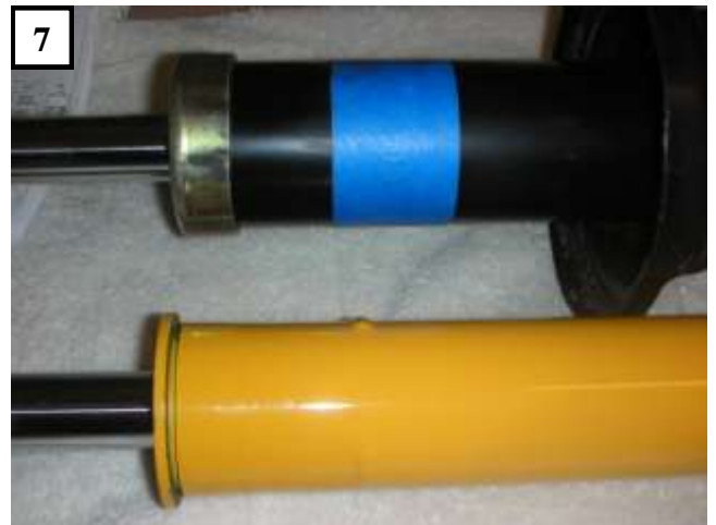
7) Mark with tape the 50mm measurement. This is where the hack saw comes into play. (remember, measure twice, cut once.)
