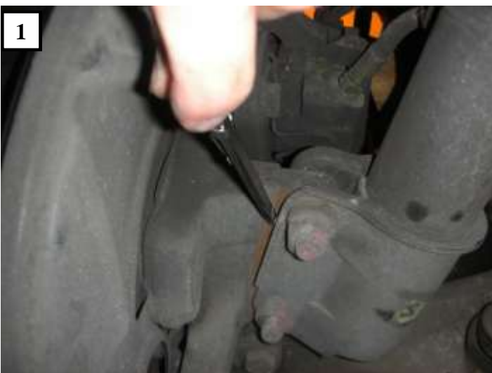
1): Using a scribe, mark the position of the old struts before removing from the car. This will help to keep the car in alignment after reinstalling—However, a professional alignment will still be necessary.
