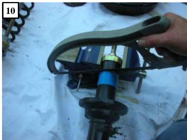
10 Here goes....Cut the strut with a hack saw at the prescribed mark (50 mm from the top)
