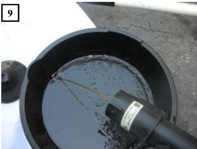
9 Drain old fluid from strut housing after drilling a hole in the bottom of the strut housing.
