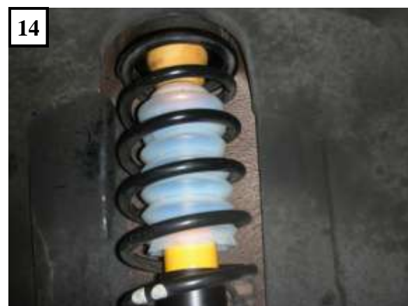
14 Installed! I also installed new 200lb springs. This will lower the car 1" and increase spring rate slightly.
