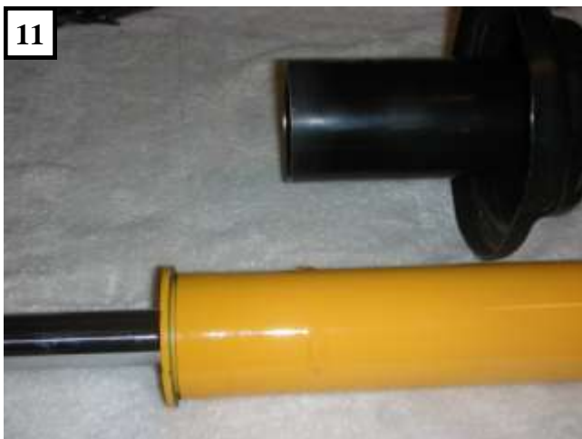
11 Compare the old housing to the new insert. The bump on the new strut will be pressed into the old housing tightly.
