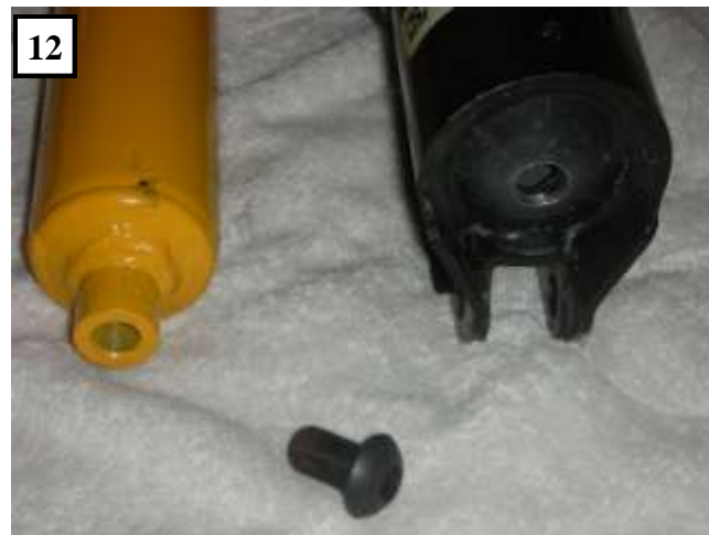
12 The new strut will be fitted into the old housing and secured with a bolt.
