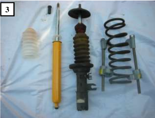
3) New Koni Strut next to old Boge Strut. The new insert will be fitted into the old housing.
