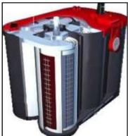
In these AGM type batteries the lead plates and the separator are wound and tightly compressed into a cell tube so they can't move, shed, or break even in severe shock and vibration applications and the separator, which is an absorbent
