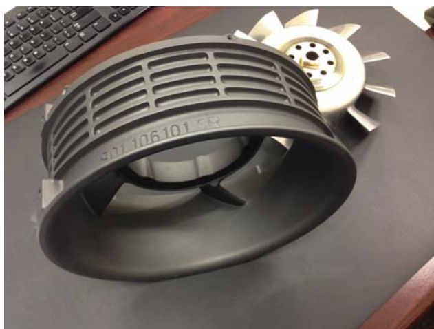
Ceramic Coated Fan Shroud and Valve Covers below
