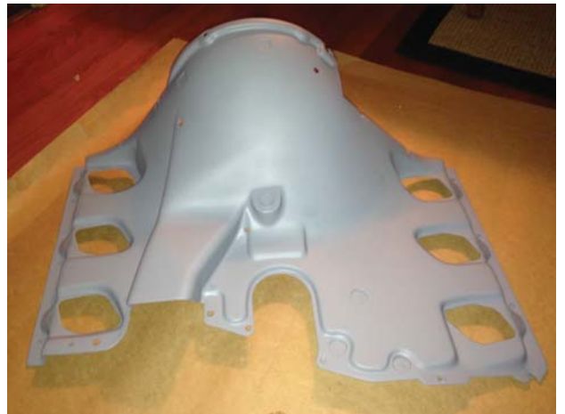
Engine Shroud after filling in scratches with Bondo and then painted with primer
