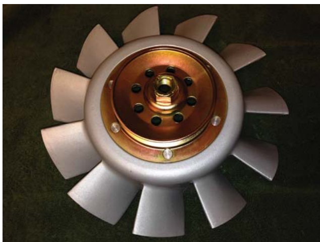
Refinished Fan and Re-plated pulley.
