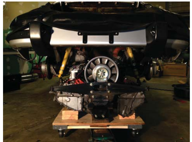
My first engine drop. Only took about an hour after building a simple platform that fit onto my floor jack.
